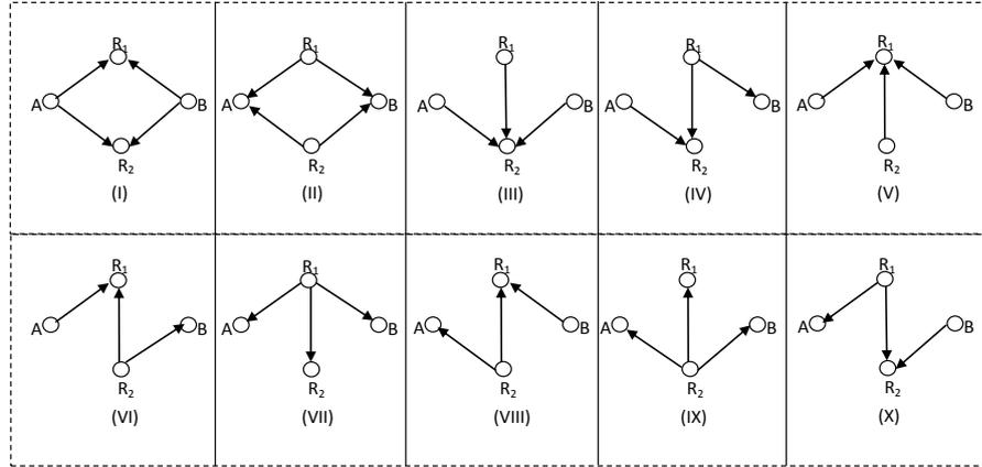
Figure 6.4: States in a Gaussian Diamond Relay network with direct link between relays.
