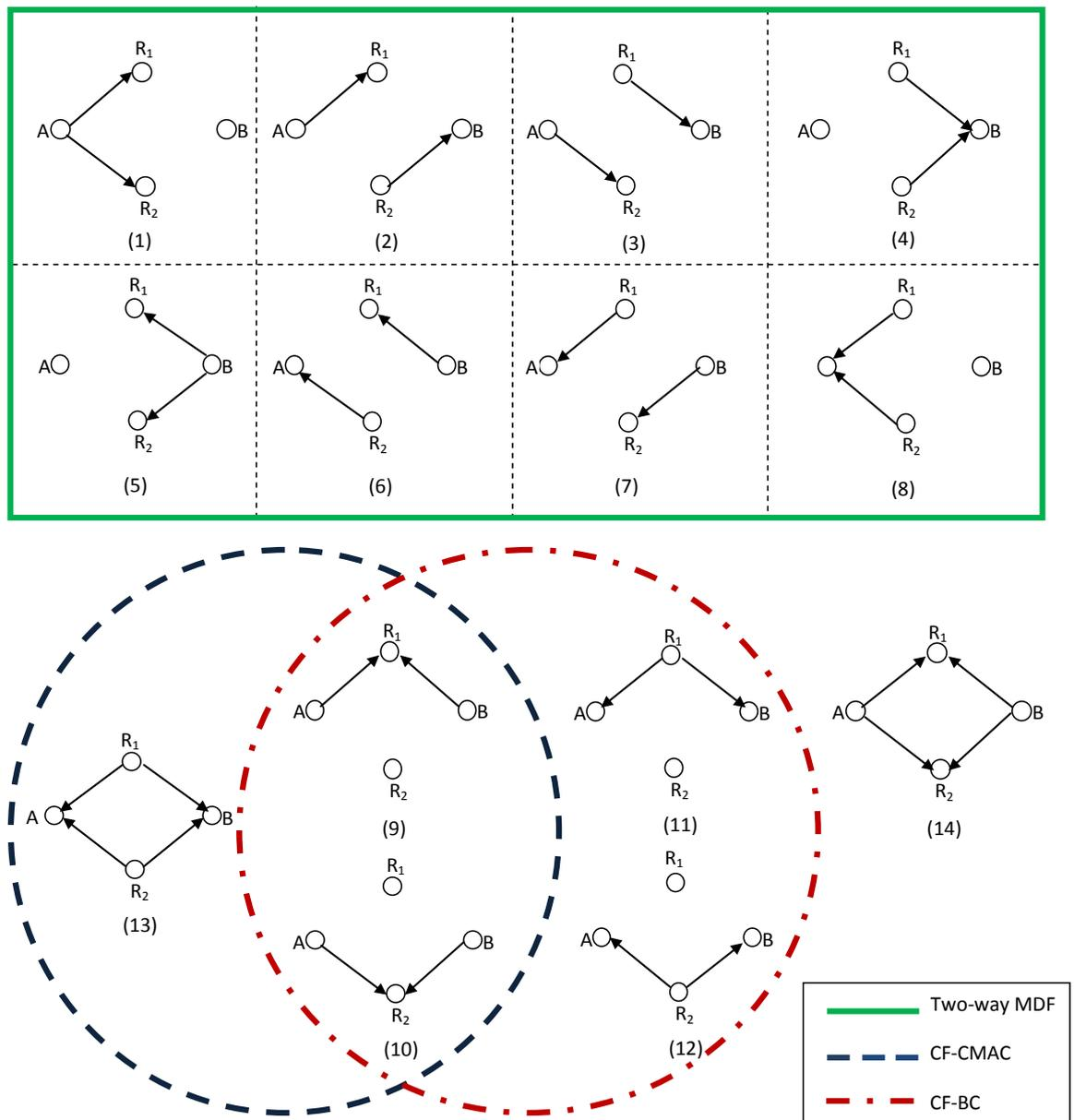
Figure 3.2: States in a half-duplex Gaussian Diamond Relay Channel
