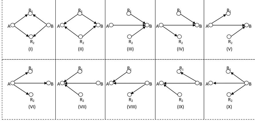
Figure 6.2: States in a Gaussian Diamond Relay network with direct link between nodes  $A$  and  $B$ .
