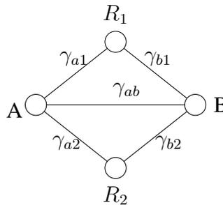
Figure 6.1: Gaussian Diamond Channel with A-B Direct Link
