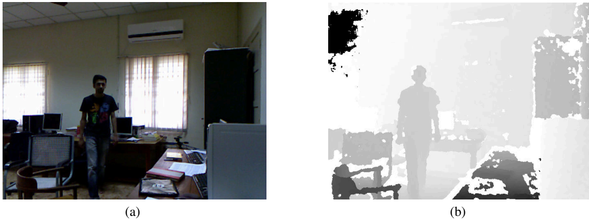
Figure 4.1: Raw result from the Kinect . 4.1a shows the color camera output. 4.1b is the depth captured from IR camera.
