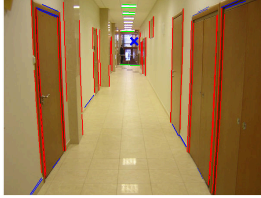
Figure 2.5: Detected line-segments, which are used to calculate the vanishing points. The three colors (red, green and blue) correspond to the line-segments for three vanishing point. One of the vanishing point is shown as a blue cross in the image. Other vanishing points are finite, but very far away in the image plane.
