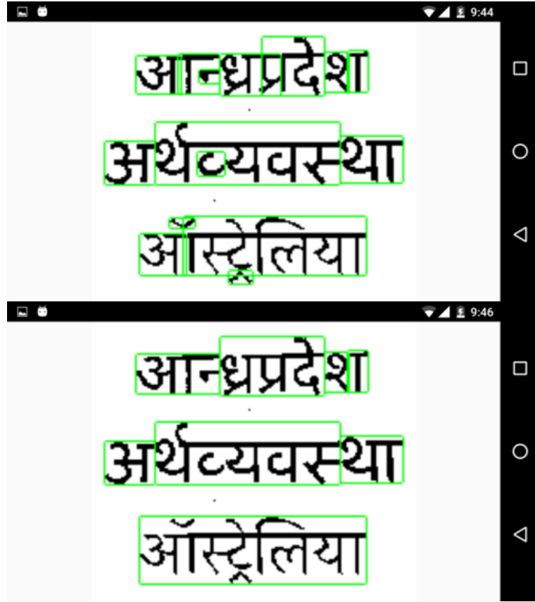
Figure 3.9: Bounding boxes after overlap merging pass
