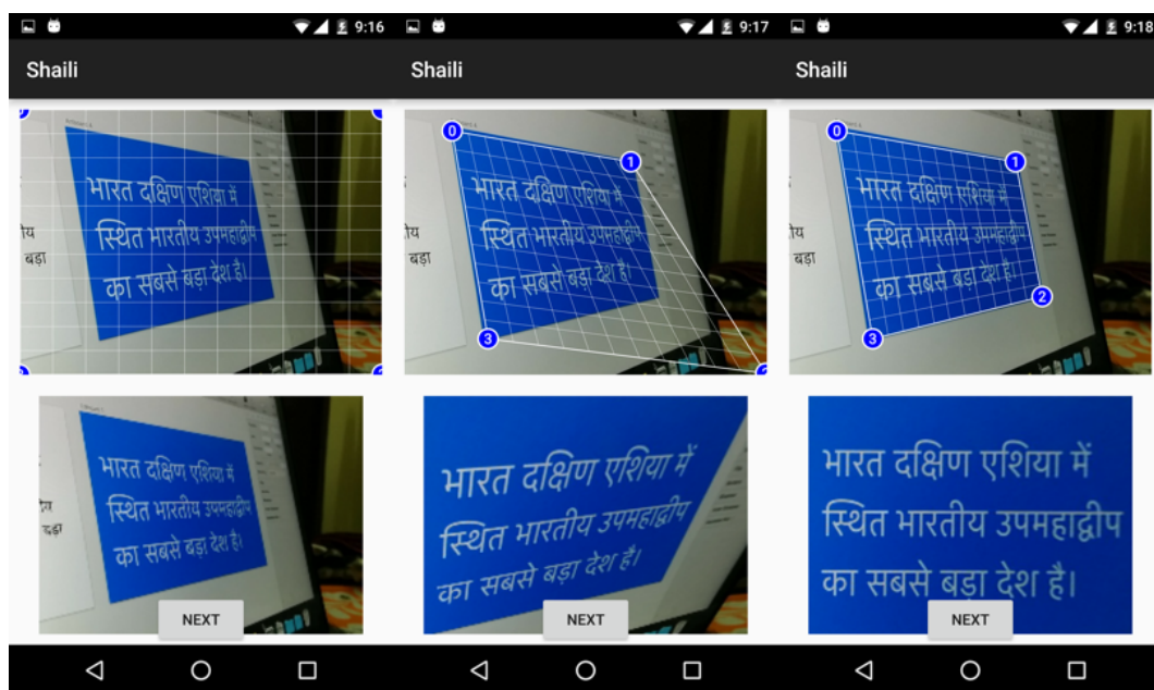
Figure 3.2: Tool for perspective cropping. The transformation is show in real-time for visual feedback to the user
