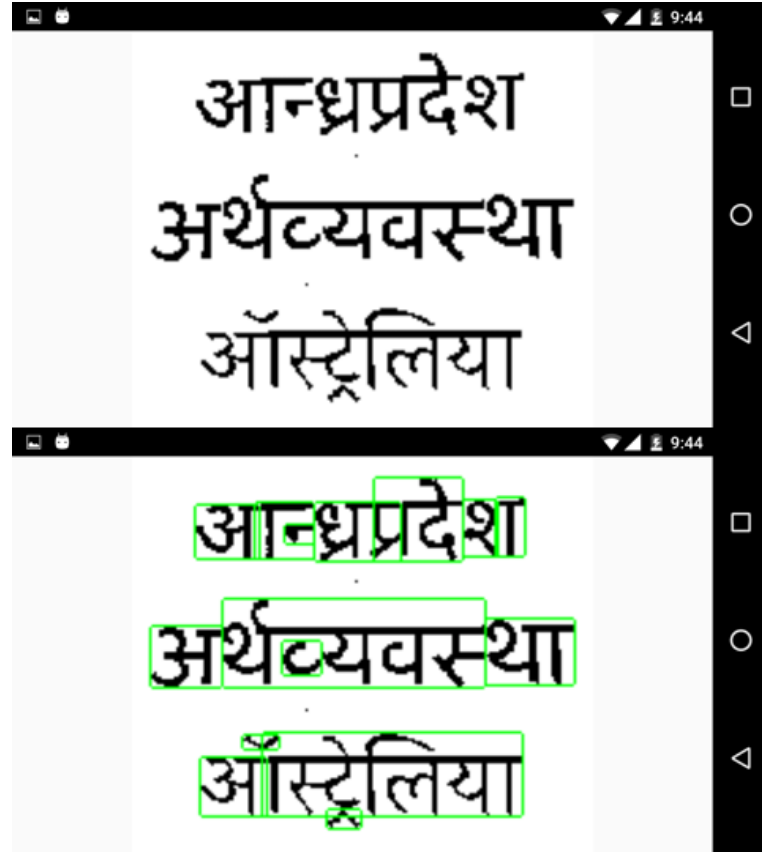
Figure 3.8: Bounding boxes obtained after Connected Component labelling
