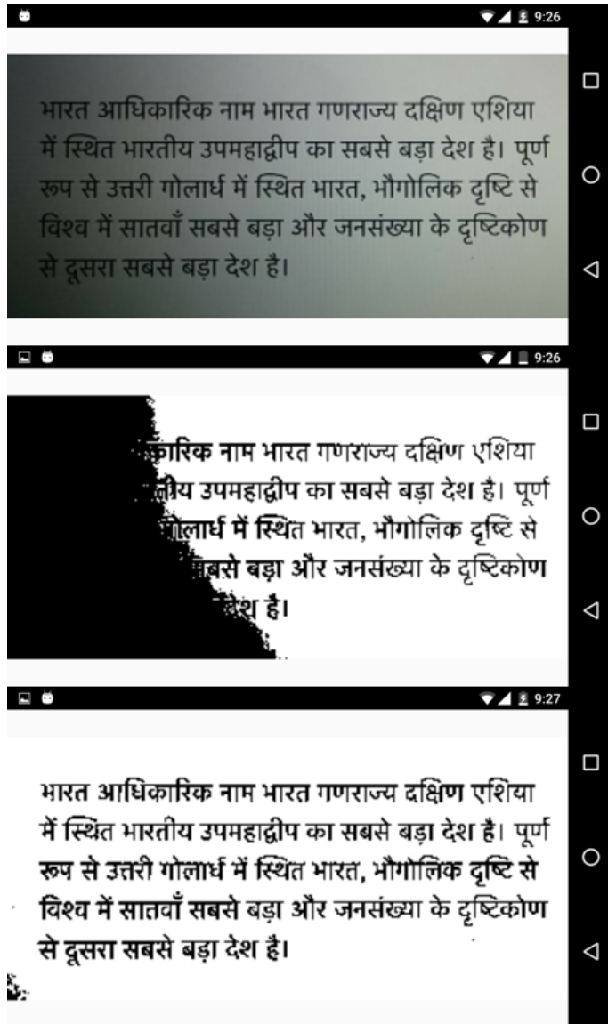
Figure 3.5: Adaptive thresholding technique compared with Otsu's method
