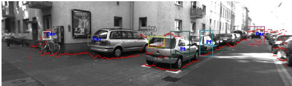
Figure 5.7: error in ground detection while car is turning right
