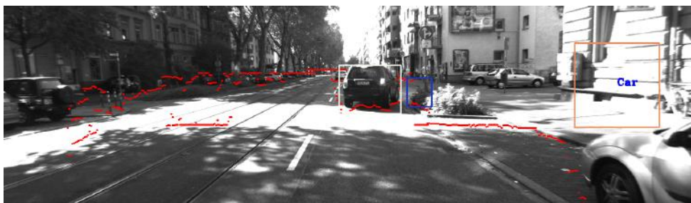
Figure 5.6: error in ground detection due to transition between shadow and bright regions.
