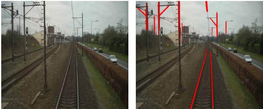
Figure 2.5: Example of lines detected by HT.
