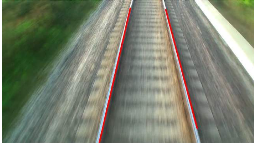
Figure 2.11: Best pair of lines detected as tracks.
