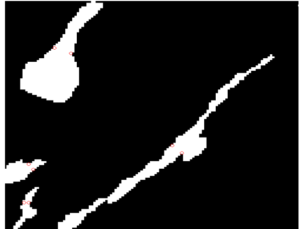
(b) A split point for the point of maximum concavity
