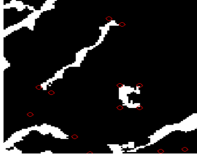
Figure 4.5: Vertices of a Rotated Minimum Bounding Box of an object
