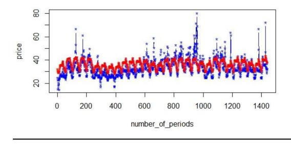
April starts with a Sunday. The first graph is the load vs the period of the day graph. The second one is the demand (red) and price (blue) vs the period of the day graph. The magnitude of demand is very high. So a reduction factor of 300 and an offset of 10 is used to reduce the demand and fit into the graph.
