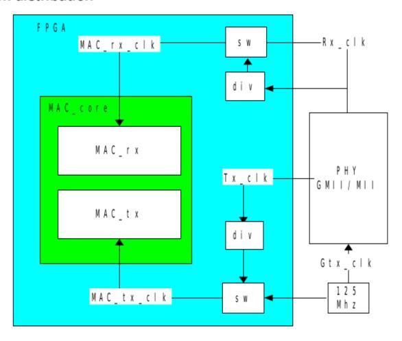
Figure 3: Block diagram of the clock distribution
