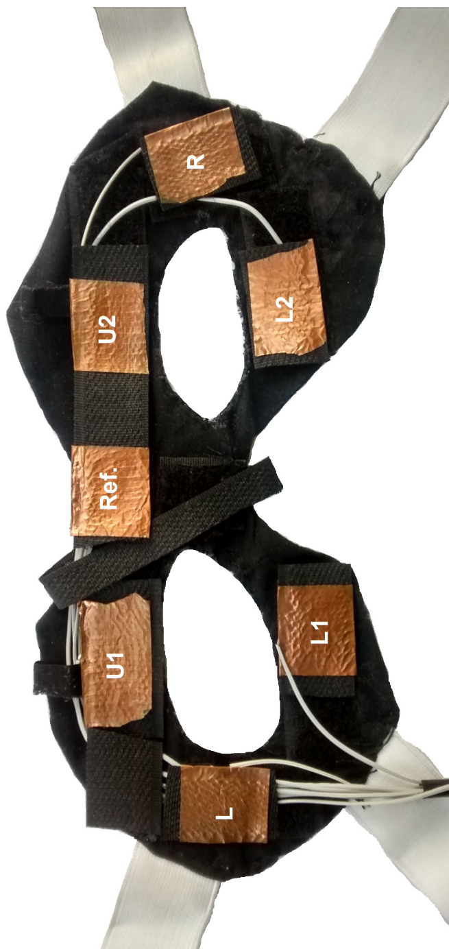
Figure 4.2: Wearable EOG mask with dry electrodes. U1 :
