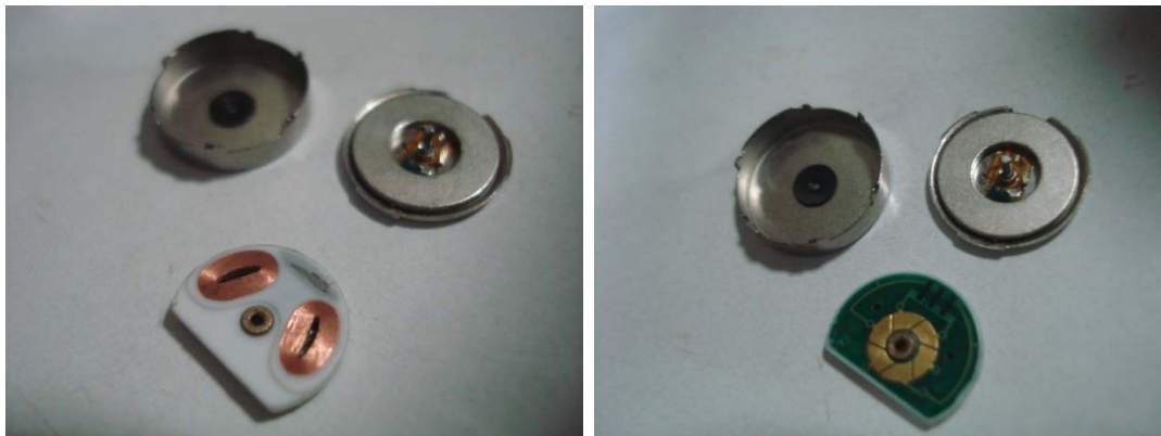
Fig 3.3.1 Mechanical Structure of ERM
