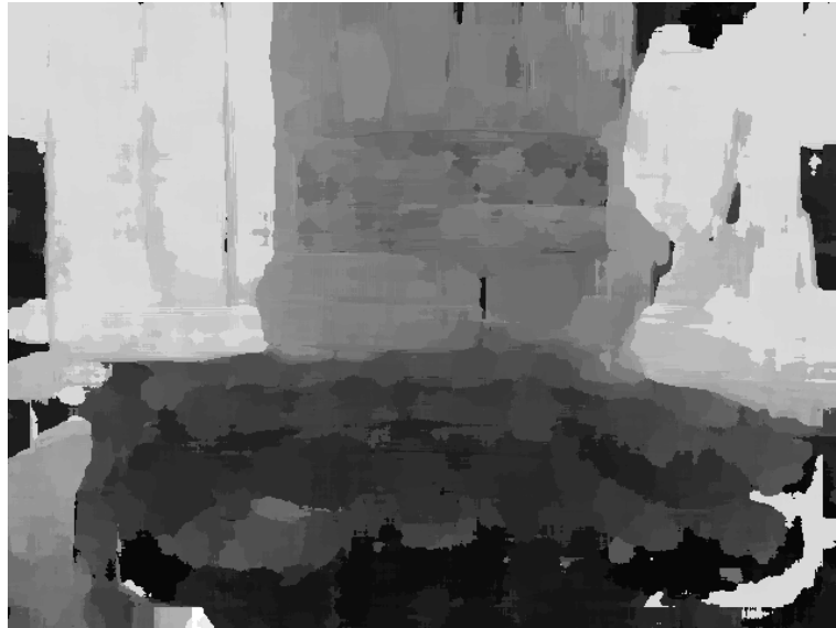
Figure 6.8: Estimated depth map. Objects nearer to the camera are darker. Observe how the objects have been segregated.
