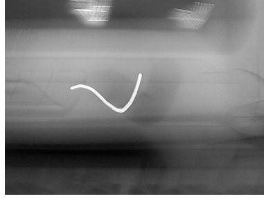
Figure 4.3: Actual image showing the point spread function, which acts as our ground truth measurement.
