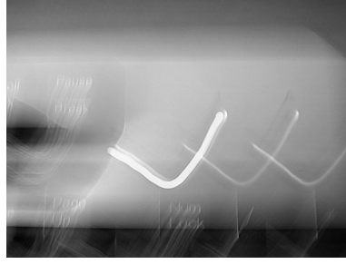
Figure 4.1: Actual image showing the point spread function, which acts as our ground truth measurement.
