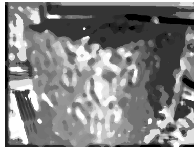
Figure 6.4: Estimated depth map. Brighter area represents scene closer to the camera.
