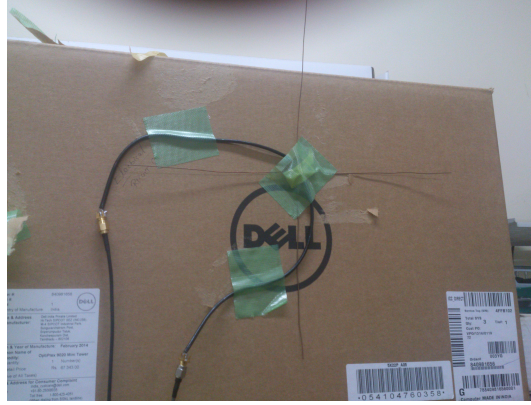
Figure 3.2: Hand made hybrid antenna
