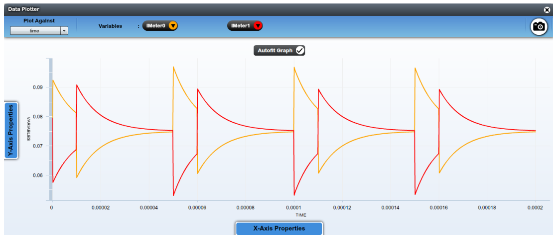
Figure 3.4: Current through LED's without using transformer @ 20 KHz
