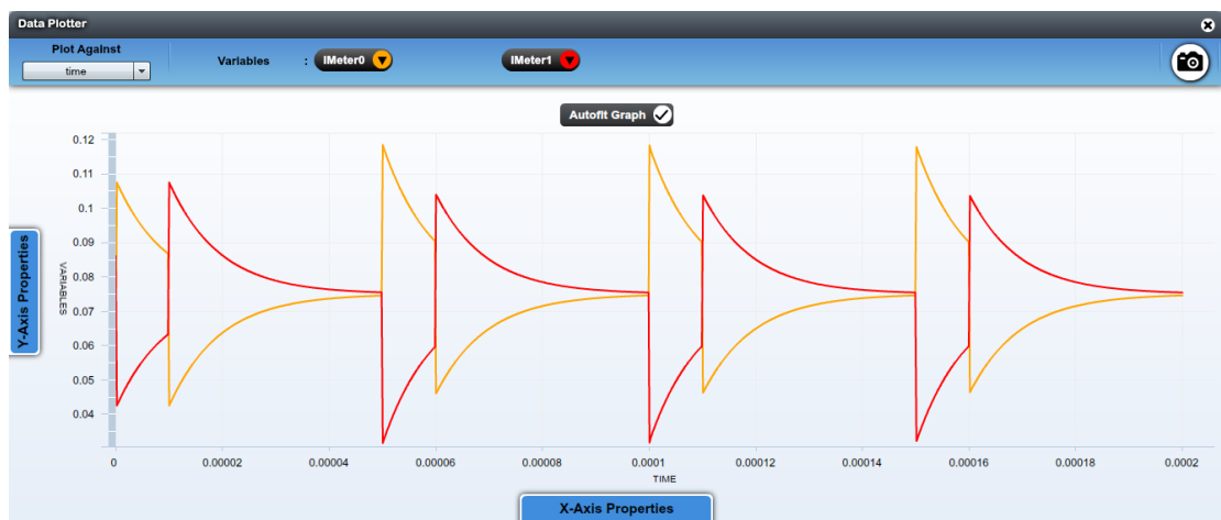
Figure 3.6: Current through LED's using transformer @ 20KHz
