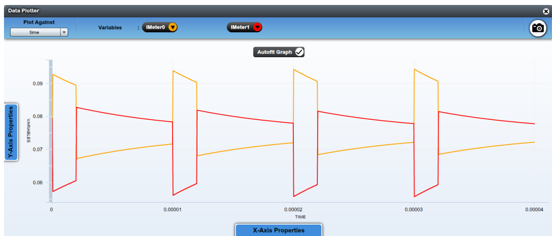
Figure 3.5: Current through LED's without using transformer @ 100KHz
