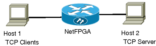
Figure 5.3: Emulation setup uses 2 Linux machines running TCP client, server and a NetFPGA hardware router. The NetFPGA router is connects through a single bottleneck link to the server.
