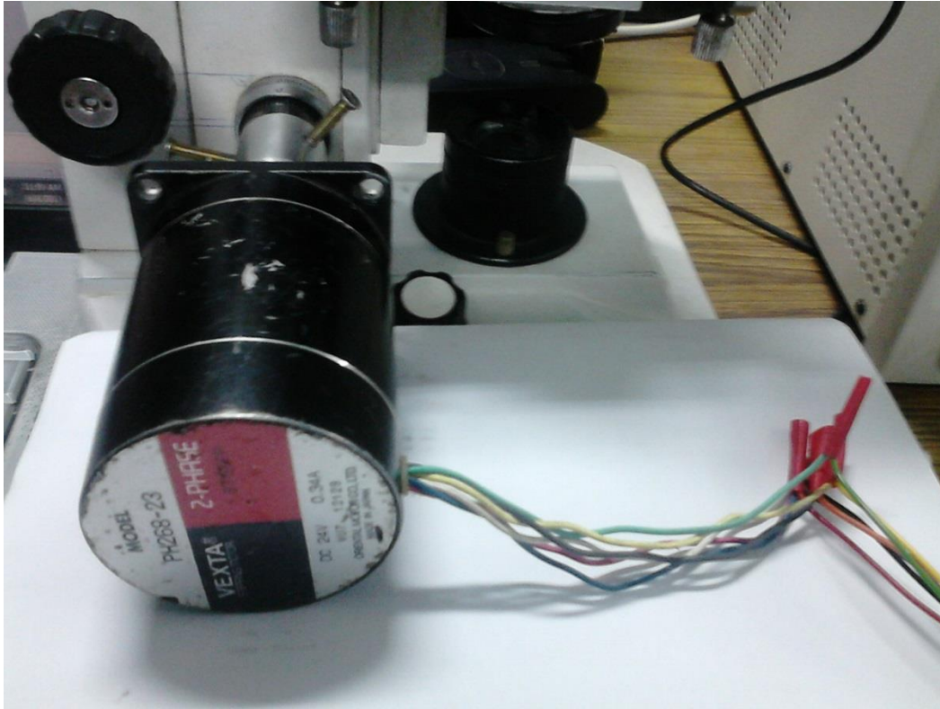
Figure 4: Stepper Motor attached to Fine Adjustment Knob
