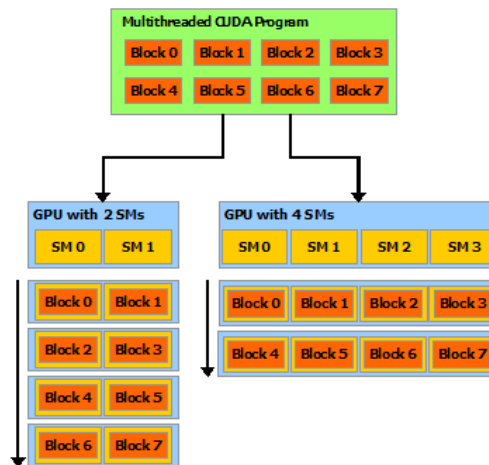
Figure 2.2: Execution model of a Cuda Program
