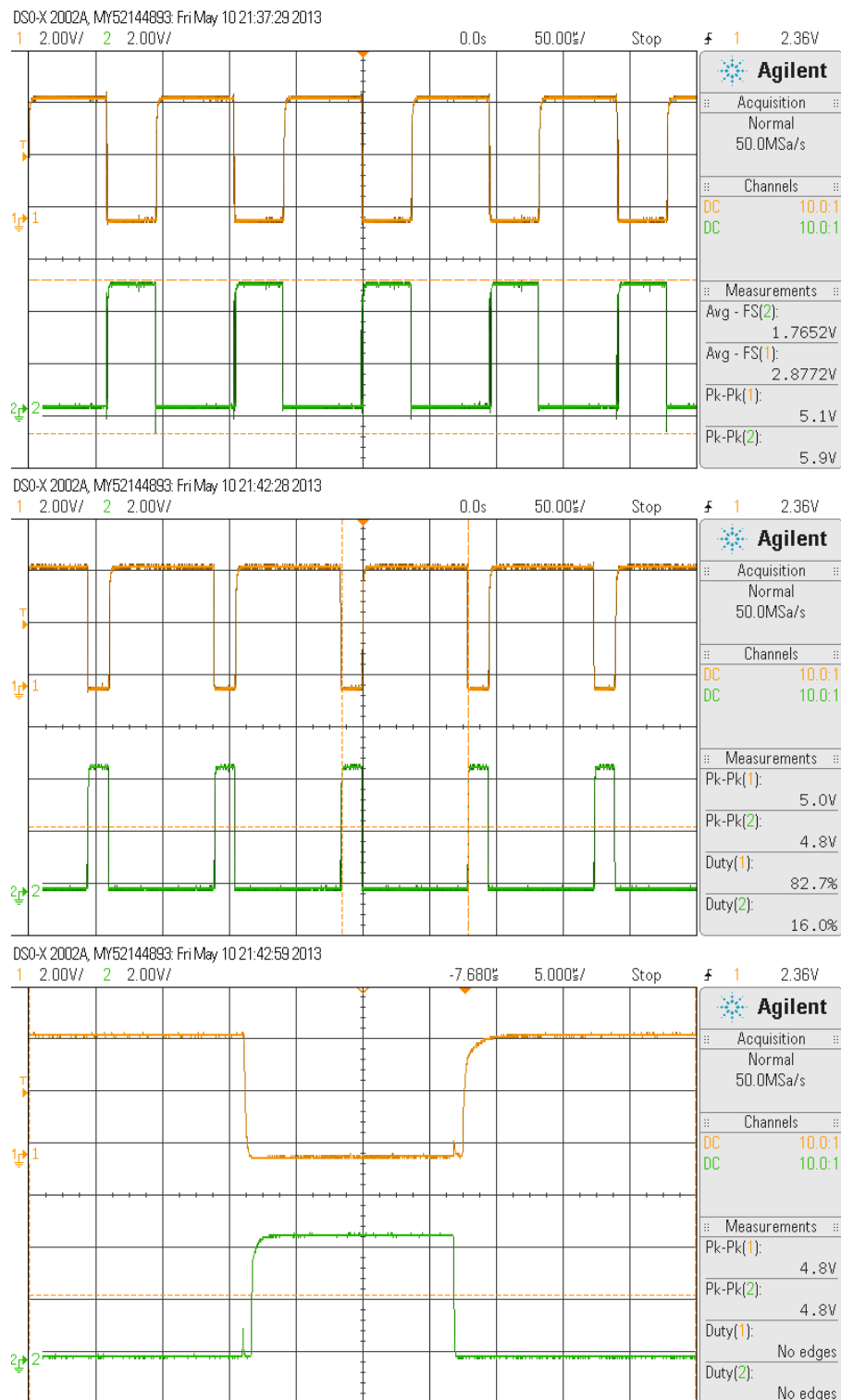
Figure 4.18: Different duty cycles from the PWM and the dead band
