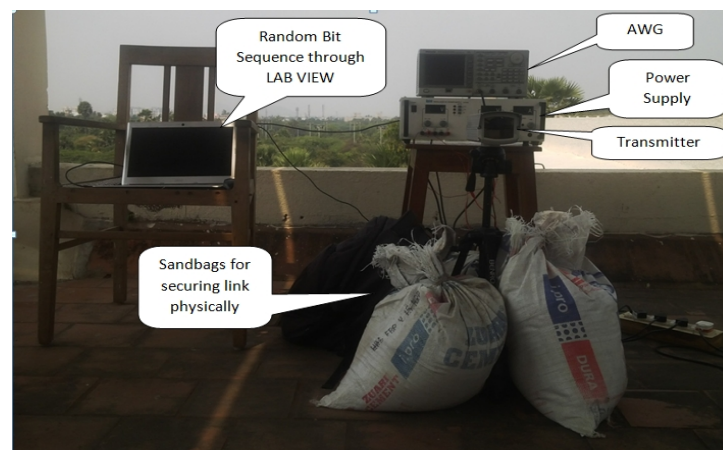
Figure 5.11: FSO Link Setup - Transmitter End
