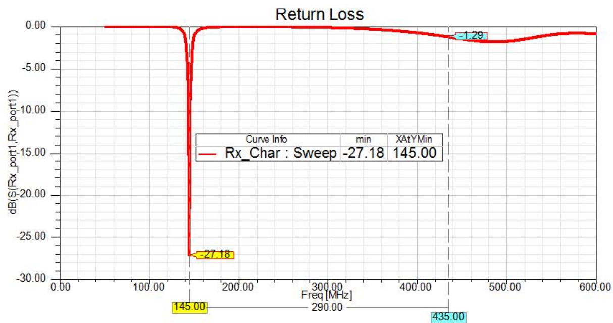
Figure 2.18.: Negative Return Loss ( S_{22} ) curves of Rx antenna
