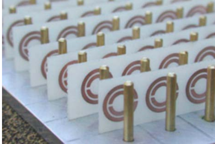
Figure 3.2: Negative refractive index metamaterial for microwaves consisting of alternating layers of thin-wire media and circular split-ring resonators (SRR).
