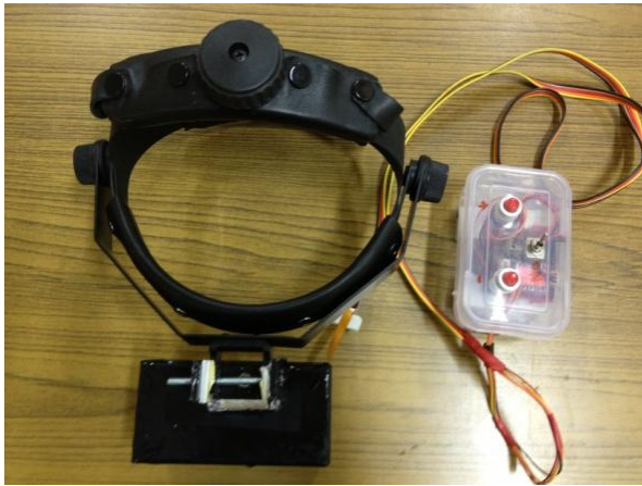
Figure 4.6(a) Head mountable prototype with control board
