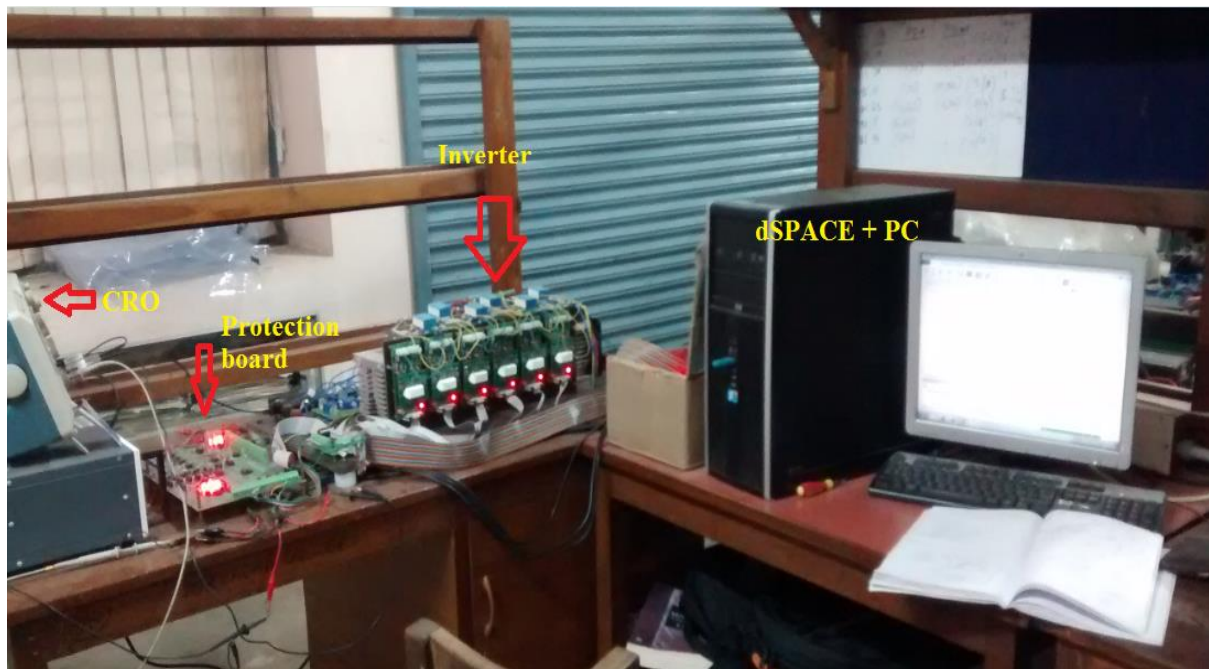
Fig 6.8: Experimental setup for 2-level-inverter fed 3 phase induction motor
